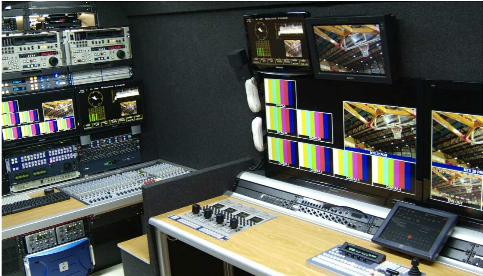
Digital 4 to 6 camera OB van • Mid-sized unit, based on a Mercedes Sprinter 316 chassis. Ideal for locations with limited space. • Ideal for general-purpose productions as sports, light entertainment, unilateral production, etc. • Dimensions: L: 710 cm, W:192 cm H 315 cm.
