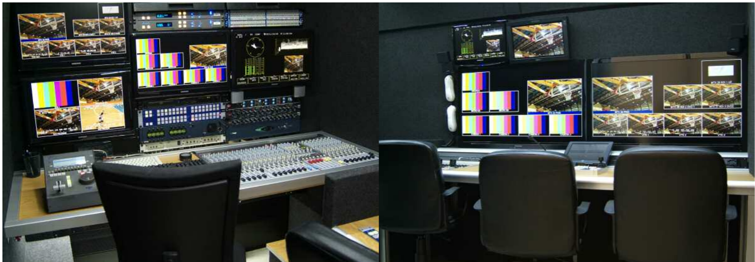
Digital 4 to 6 camera OB van • Mid-sized unit, based on a Mercedes Sprinter 316 chassis. Ideal for locations with limited space. • Ideal for general-purpose productions as sports, light entertainment, unilateral production, etc. • Dimensions: L: 710 cm, W:192 cm H 315 cm.
